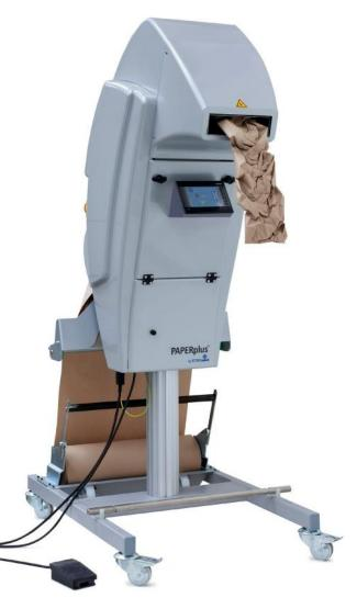
PAPERplus® Classic<sup>2</sup>, the new machine model from Storopack, processes rolls of Kraft paper and recycled paper into paper padding for protective packaging of medium-weight to heavy-weight products.
